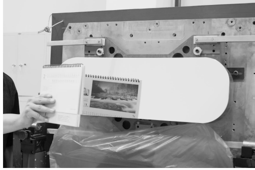
图 7 表面改性非球面碳化硅反射镜抛光后的实物照片 Fig. 7 Photo of surface modification aspheric SiC mirror after polishing
